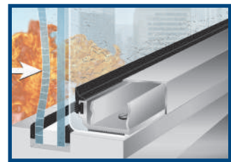
Blast impact shatters external glass and drives it against the inner pane.
